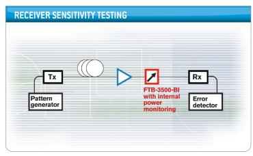
Figure 2. Typical receiver sensitivity setup
