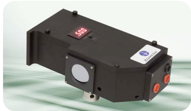
Figure 12. ZAP-APD picture showing the THz input window.
