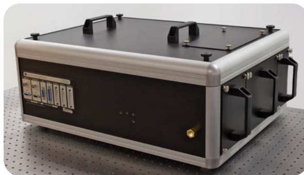
Figure 6. Picture of standard Z3 THz TDS. The pump beam enters (external laser not shown) in the rear of the spectrometer and the purgeable system has three ports on the front to send the terahertz beam as required by the application. Control of the Z3 is enabled by TAC software and the connector bus shown above.
