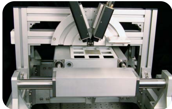
Figure 2. FiCO heads mounted on integrated imaging stage in pitch-catch geometry. Transmission and normal reflection geometries are also possible with this imaging stage.
