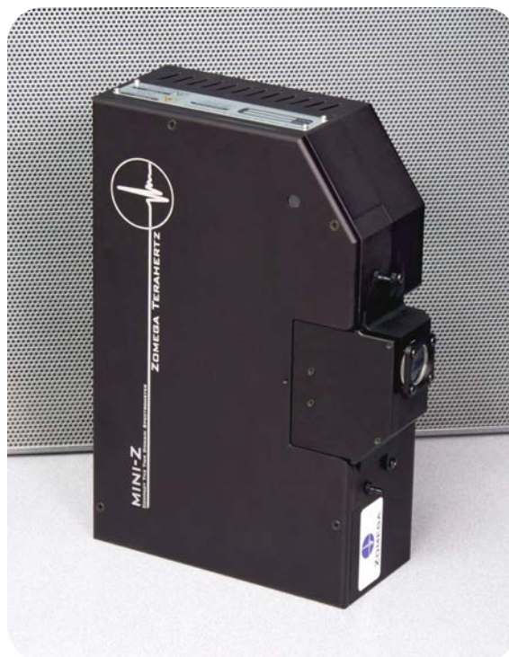
Figure 4. Mini-Z with the normal reflection module mounted. Mini-Z includes both transmission and reflection modules.
