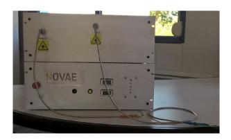
Coverage is a turn-key supercontinuum source emitting a continuous spectrum from 1.9  $\mu$ m up to 4.0  $\mu$ m. The very high brightness associated to the high average power allows a wide range of applications such as spectroscopy, spectro-microscopy or optronic counter-measures.
