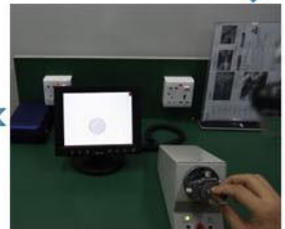
Cleaning end face
