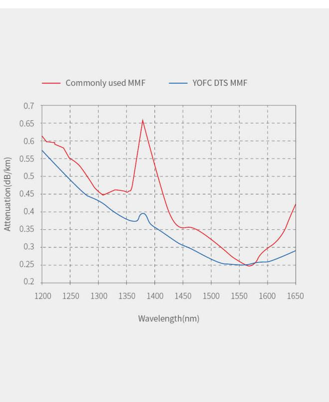
**Compared with communication multimode fibre, the advantages of DTS-MMF are as follows:**
