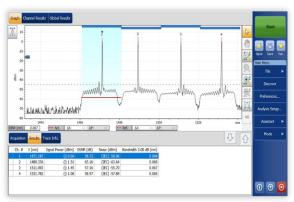
The FTBx-5235 displays channel power, channel wavelength and OSNR. Above: example of CWDM network OSA display.
