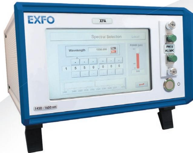
The XFA is electronically controlled and wavelength tuning ranges from 1450 nm to 1650 nm. The bandwidth is factory-set and can be selected at purchase between 50 pm and 800 pm with respect to the center wavelength.
