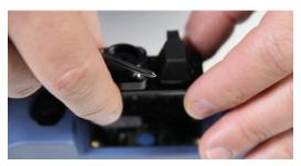
The power meter and VFL piece are offered as an easy-toinstall option on the MAX-FIP display that's as simple removing four screws.
