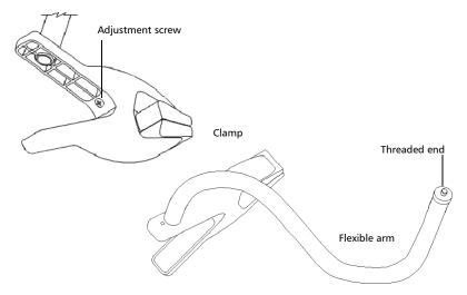
**3.** Using the threaded hole on the back of the TG-300B, screw it on the end of the flexible arm.
