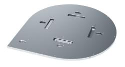
Heat sinking platform can be used to coil the T-DCF and mount the components (CMS and splice protector) securely. For high-power operation the heat sinking platform needs to be mounted onto an actively cooled external heat sink.
