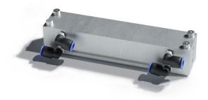
Water-cooled fiber holding block allows direct water-cooling of the T-DCF's tip, which has the highest heat load under pumping. This fiber holder can be easily mounted onto a translation stage, making the aligment procedure easier.
