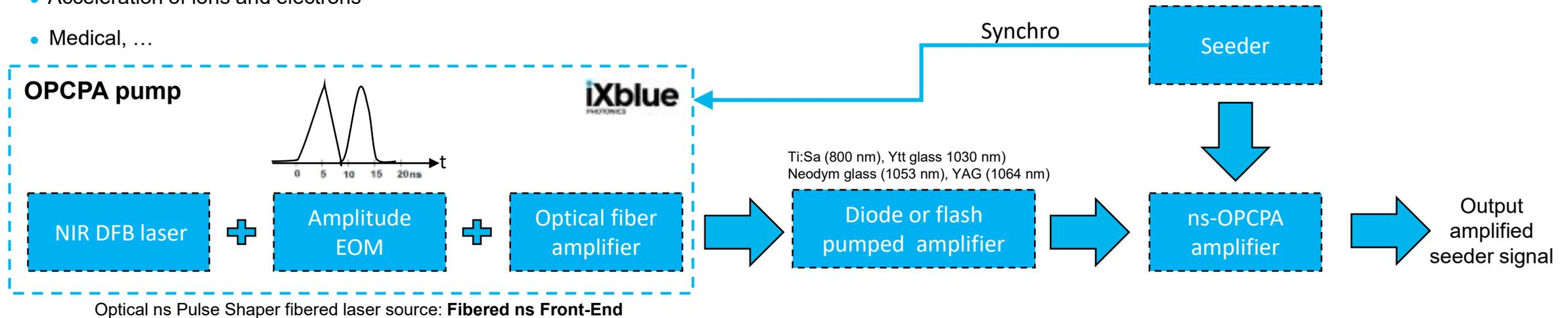
• OPCPA pump source - key LiNbO<sub>3</sub> modulators specification:
