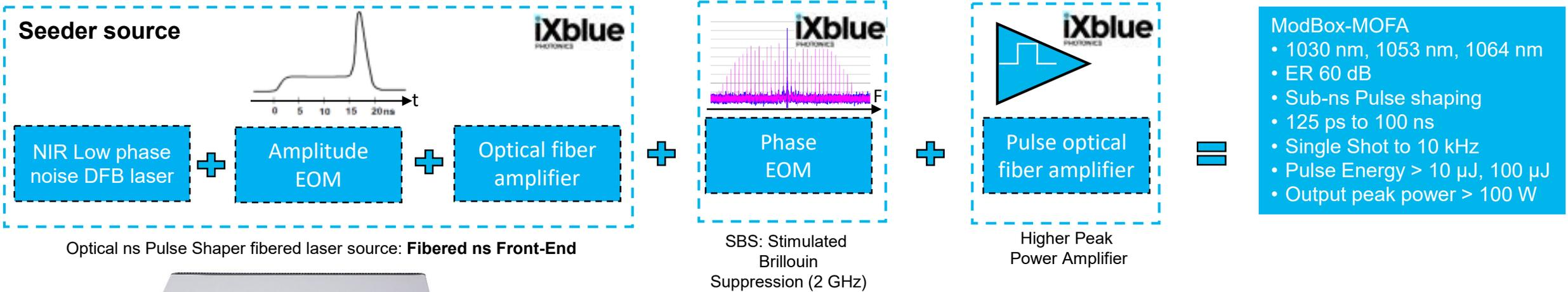
Optical ns Pulse Shaper fibered laser source: **Fibered ns Front-End**
