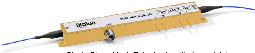
Single Stage Mach-Zehnder Amplitude modulator
