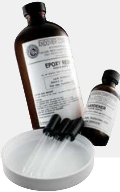
Fuller Epolite FH-5313 is a 100% solid, room-temperature curing, optically clear, electrical grade epoxy. Proven to be a superior bonding agent for ferrite pot cures, this system is designed for continuous operation at temperatures up to 200°F. Resin and hardener are sold individually or in kits, and in pre-measured A-Paks.
