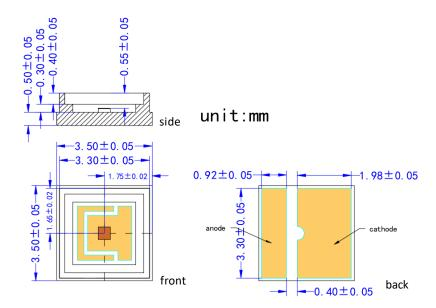
VD-0940V-003W-1D-2B0 with Substrate 1=AIN and Package D=5050 (unit: mm)
