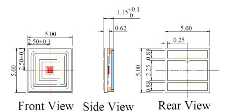
VD-0940V-003W-3E-2B0 with Substrate 3=Cu/Ag and Package E=7060 (unit: mm)
