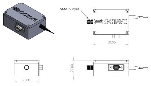
Dimensions are in millimeters. The SMA connector provides RF output from detector. The Micro-D connector provides connections for detector power (5-15 VDC, ~0.6 W), thermistor, and built-in thermo-electric cooler.
