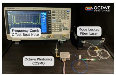
**Customization:** The COSMO can be customized to meet specific requirements. In the photo, a miniaturized version of the COSMO (the COSMO-mini) has been constructed to keep the size and weight to a minimum. The COSMO-mini does not contain the electronic amplifier, and instead provides direct electronic access to the photodiode. The COSMO can be provided in other form factors as applications require.
