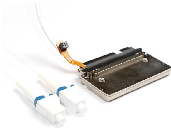
Beogold Technology CFP2\_EDFA can be flexibly integrated into various DCO modules in CFP/CFP2/QSFP-DD/OSFP enclosures to meet various customization needs of customers. It can maximize space utilization, effectively compensate for the insertion loss of various optical devices in space- and power-limited DCOs or transponders, and work in the full C-band for single-wavelength optical power amplification.
