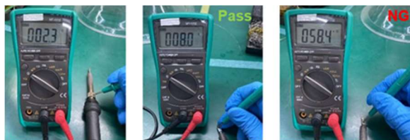
Figure 4 - Soldering tool resistivity check 焊接工具电阻检查
