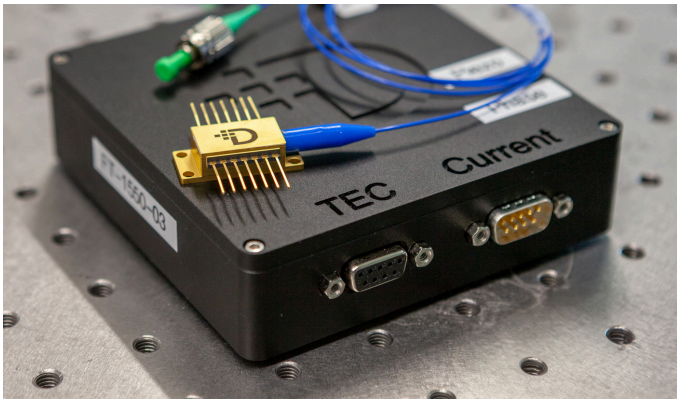
Laser head. The controller ready head, with its temperature and current connectors, and a butterfly module on the lid.
